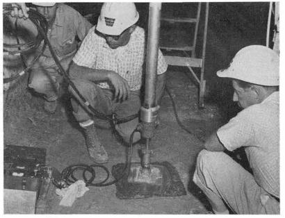
SHOCK WAVE MEASUREMENT — Three Sandia Corporation employees, Carl E. Smith, left; Austin C. Arthur, center, and H. M. Miller (all 7254), check hydrodynamic gauge which will be used in measuring speed of shock wave produced by nuclear explosion during Project Shoal experiment Oct. 26 near Fallon, Nev. The gauge is one of many located along shaft leading to the detonation point 1200 ft. underground.
